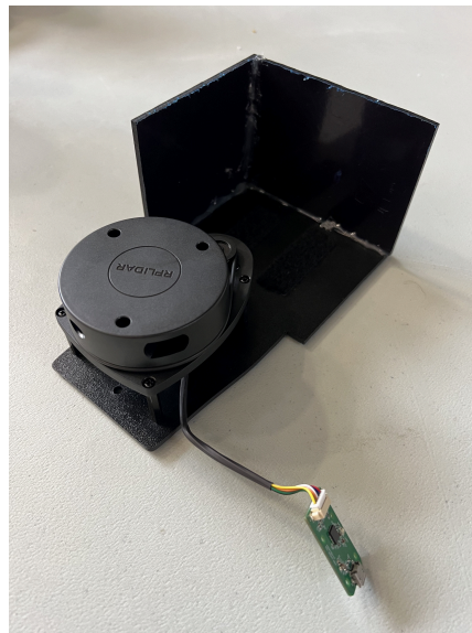
Figure 13: LiDAR fastened on the Mount
